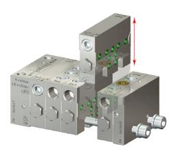
nPr+ uses an innovative "rail & lock" concept to allow the element to be replaced or moved without the need to completely dismantle the assembly. This is an industry first for segmented progressive dividers allowing quick easy modification or replacement of an assembly element without the cost of separating from the base.
